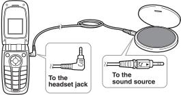
1) Connect the audio recording cable to the handset and sound source (e.g.stereo or cd player). Insert one end of the audio recording cable into the handset's headset jack and the other end into the sound source.
